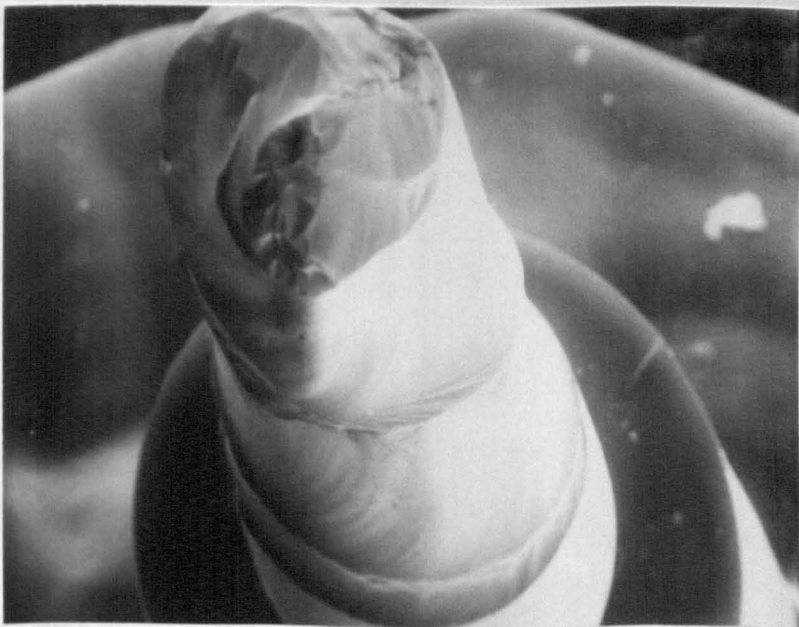
FIGURE 23: Fractograph of optical fibre failed under combined tension and torsion due to internal flaw.
