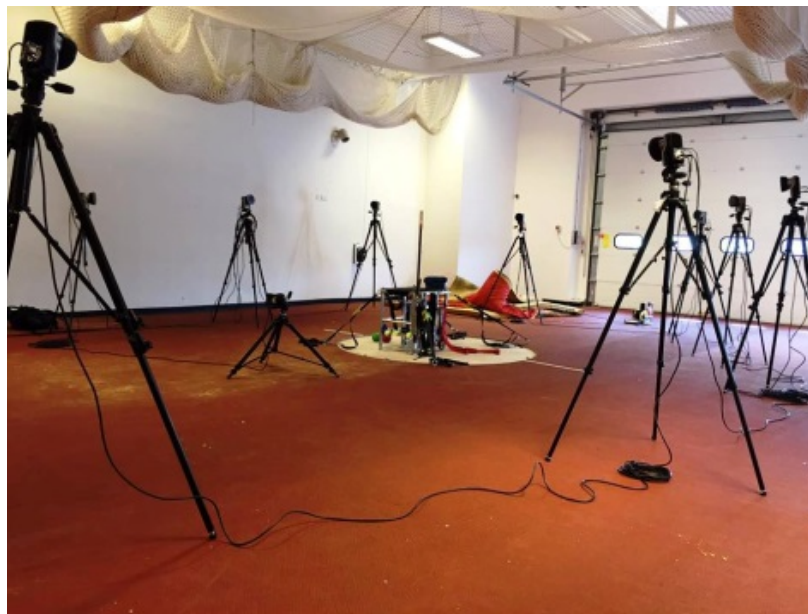
Figure 4 4: Testing set up showing participant's diagonal seating position (front leg facing forwards and back leg facing diagonal to right side) and 10 cameras situated around the throwing area.
