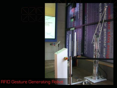
The installation invites visitors to touch a suitable RFID card, such as an Oystercard, against a reader and then generates a unique and repeatable gesture in space according to the serial number of the card, in a movement reminiscent of a conductor's baton or magician's wand. It explores the representation of data using physical movement and the generation of elegant motion.
