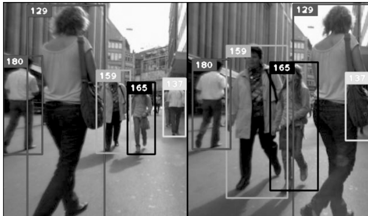
Figure 42. Illustration of bounding boxes for motion tracking
