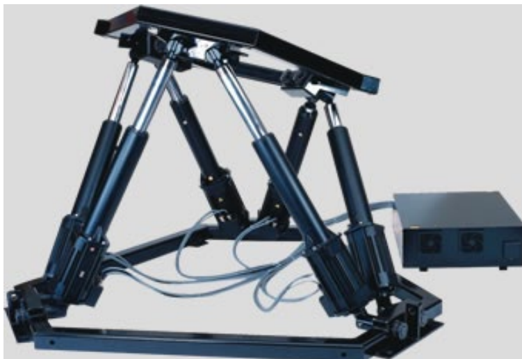
Figure 30. illustration of a motion base robotic platform courtesy of W.S.Harwin, Reading University.
