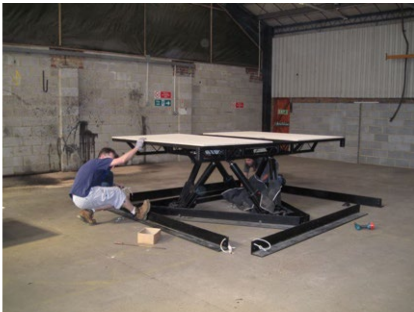
Figure 31. Gravity Shift research and development showing the Motion Base with stage platform construction.
