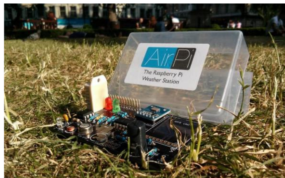
Fig. 1 - AirPi - A Raspberry Pi based weather station
