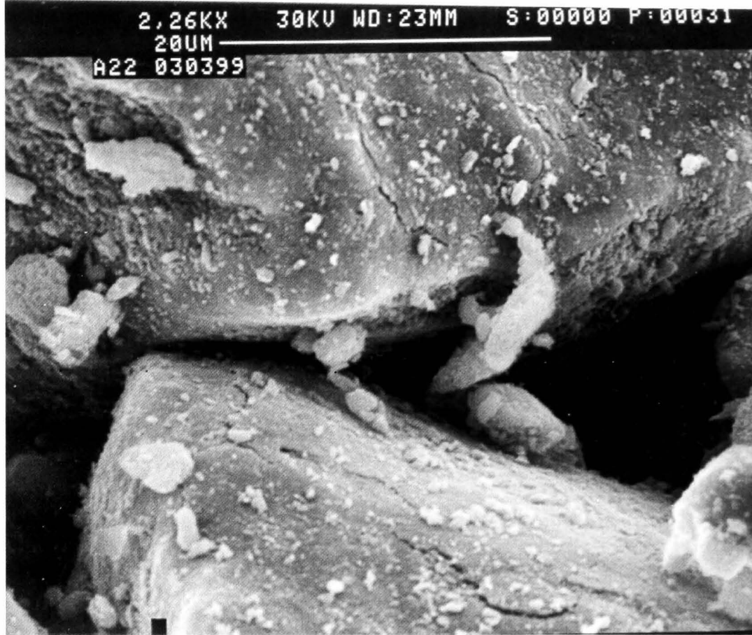
Fig. 3.34 SEM picture of H-inserted SBP-A in the homogeneous region ( s = 0.143 ) at medium magnification. Note the limited cracking of the particles.
