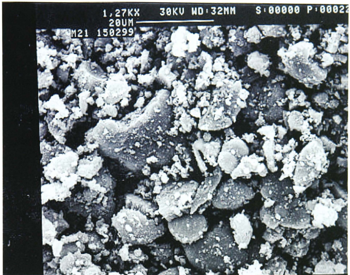
Fig. 4.29 SEM picture of H-inserted Faradiser M ( s = 0.564 ) in the first homogeneous phase at about \frac{1}{2}M . Particles are further cracked and broken.
