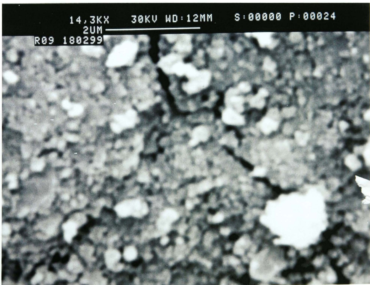
Fig. 5.38 SEM picture of a particle of H-inserted R2 near the start of the first heterogeneous phase ( s = 0.408 ). High magnification shows that the particle was cracked.
