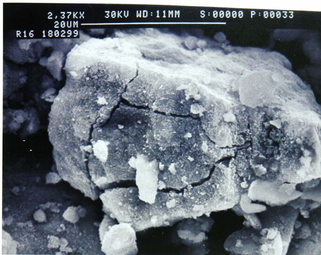
Fig. 5.39 SEM picture of a particle of H-inserted R2 near the end of the first heterogeneous phase ( s = 0.624 ). Medium magnification was enough to reveal the severe cracking.
