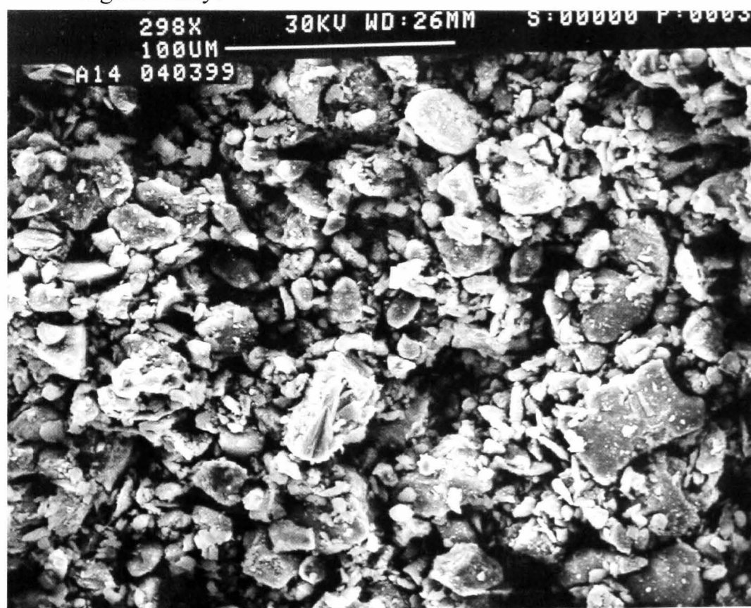
Fig. 3.36 SEM picture of H-inserted SBP-A in the heterogeneous region ( s = 0.589 ) at low magnification. Note that the particles size has reduced significantly.
