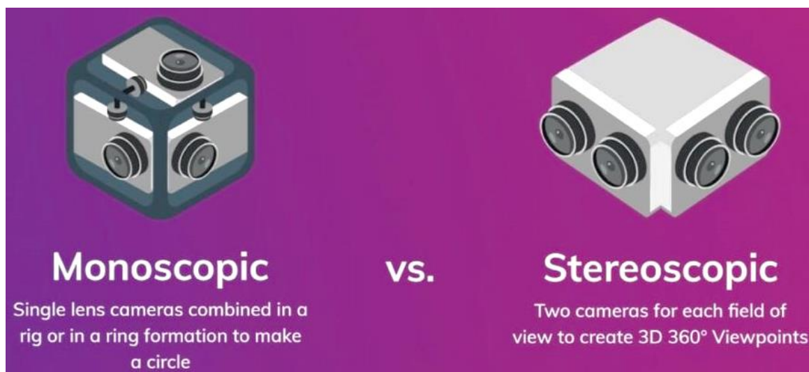
Figure 2.14: Monoscopic and stereoscopic 360° cameras differences (VRdirect, 2019).
