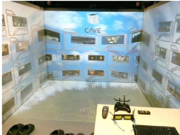
Figure 2.6: A VR CAVE, glasses and Xbox controller (Matsentidou and Poullis, 2014).
