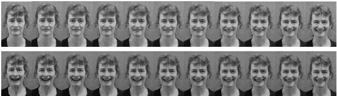
Figure 27: Sequence of interpolation of facial emotion: sad to happy and scared to happy
