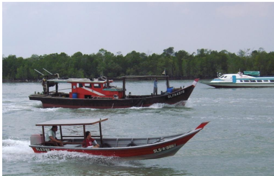
Photo 4.10. Comparison of sheer lines. Open boat in foreground, Class B fishing boat in middle, modern high speed, steel passenger boat in background. Pulau Ketam.
