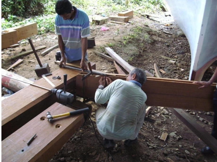
Photo 5.3. Producing the stem post and keel bar connection. Kuala Terengganu.
