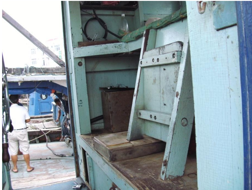
Photo 4.17. Typical helm with seat folded up. Pontian Kecil.
