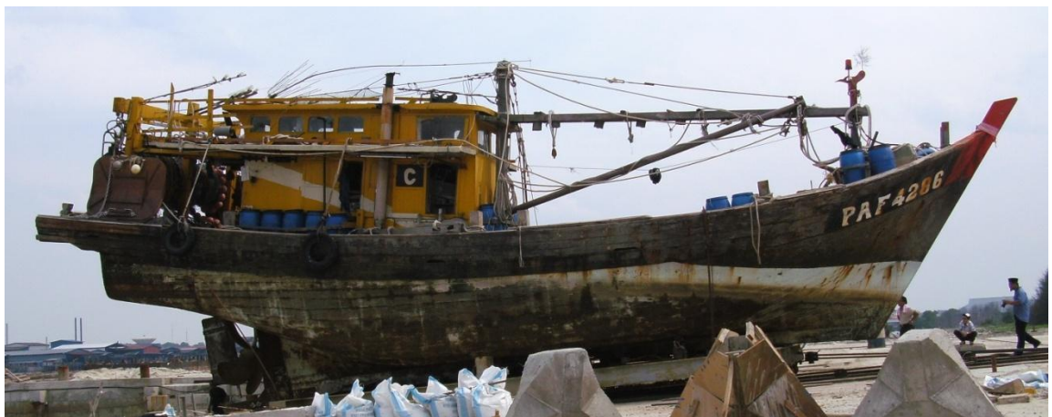
Photo 5.1. Overhung transom, Class C trawler, approximately 20 years old. Mersing.
