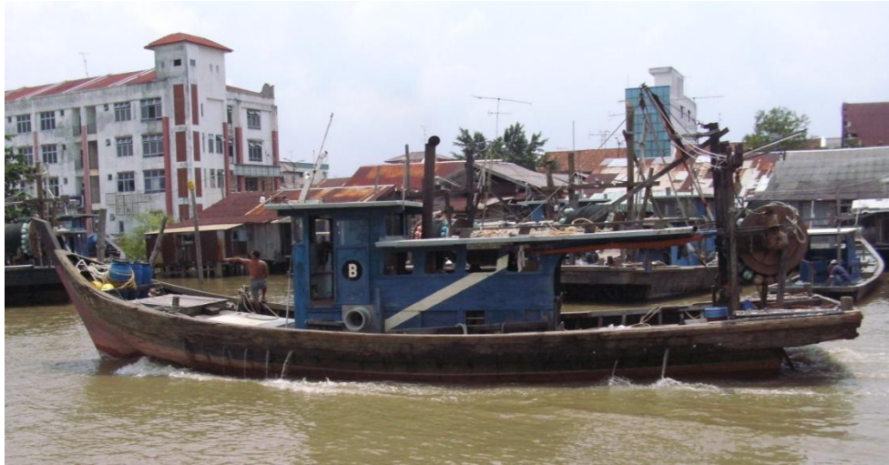
Photo 4.6. Freeing ports draining water from deck washdown. Pontian Kecil.
