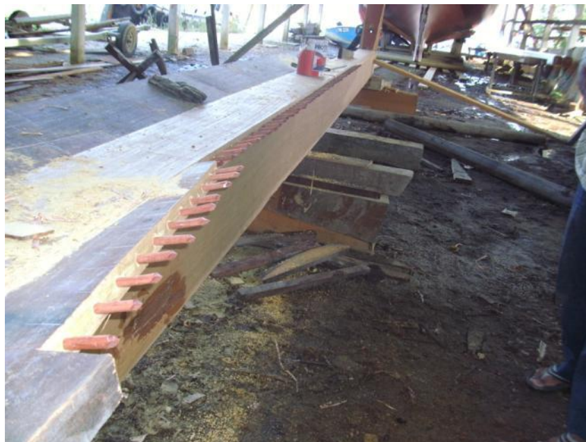
Photo 4.25. Elaborate use of trunnels to produce monocoque hull. Kuala Terengganu.
