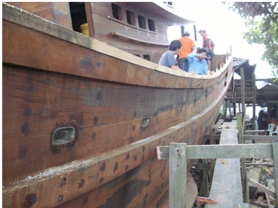
Photo 4.5. Freeing ports on new Class B fishing boat surveyed in Kuala Terengganu.
