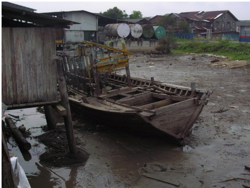
Photo 4.13. V shaped cross section towards bow. Endau.
