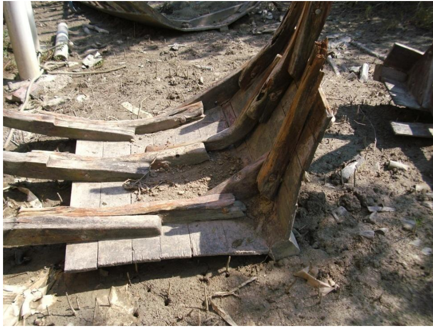
Photo 4.15. Remnant of U shaped hull showing framing construction. Pulau Ketam.
