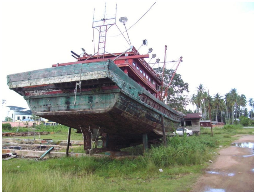
Photo 4.16. U shaped hull section. Tumpat.
