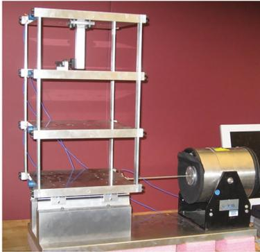
Fig. 5. Three-story frame structure experiment [24].
