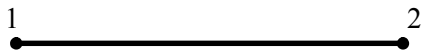
Figure 1.2: A one-dimensional linear finite element consisting of two nodes. The interpolation function is a simple linear relationship for the dependent variable along its length.
