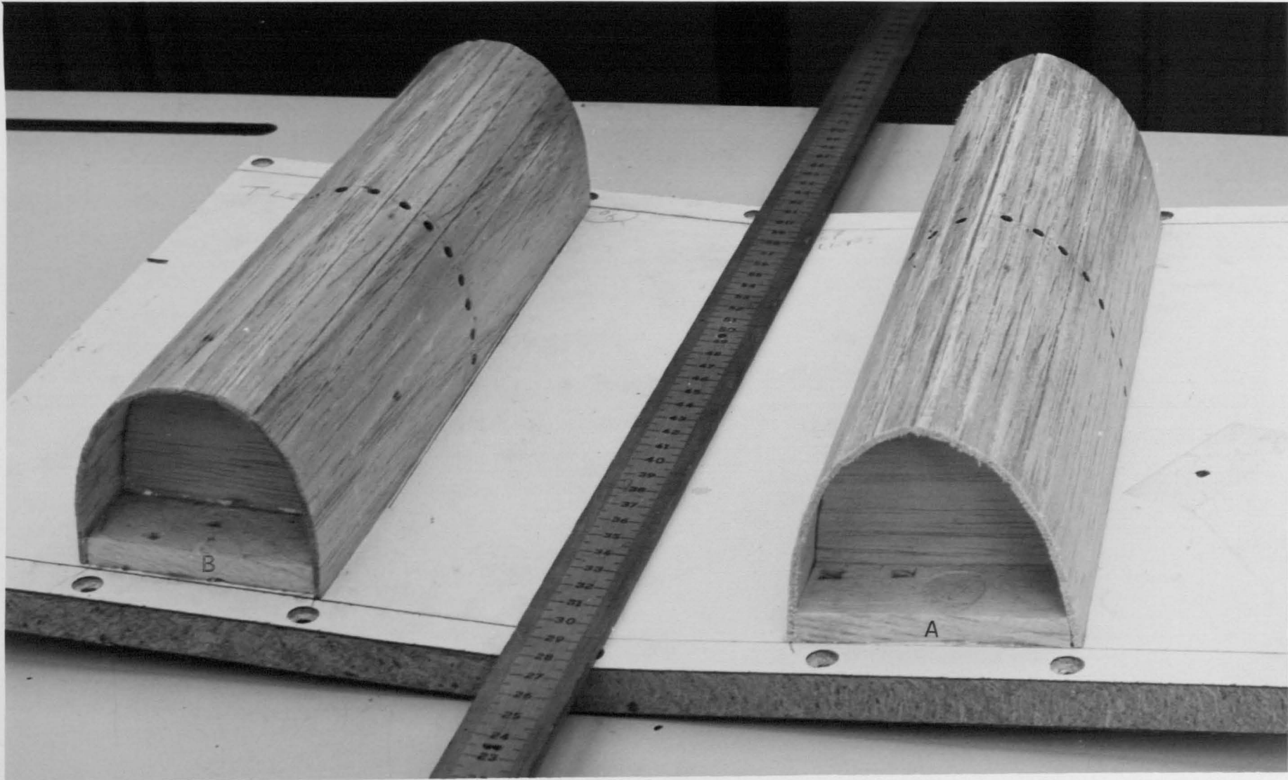
Photo 1. The semi-elliptical cylinder model (A) and the scaled model of the proposed structure (B) for the current experiment.
