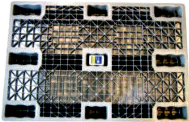
Fig. 1.12. Sensor plugged inside a Pallet.
