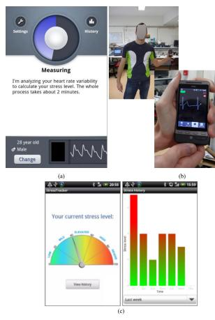
Fig. 6: Android apps for measuring stress, with and without additional hardware: (a) Stress Check, (b) Droid Jacked [73] and (c) Stress Tracker [74].
