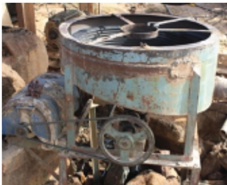
A simple centrifuge concentrator
