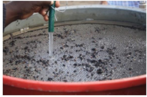
The milled ore being screened and fed into the bowl below by running water
