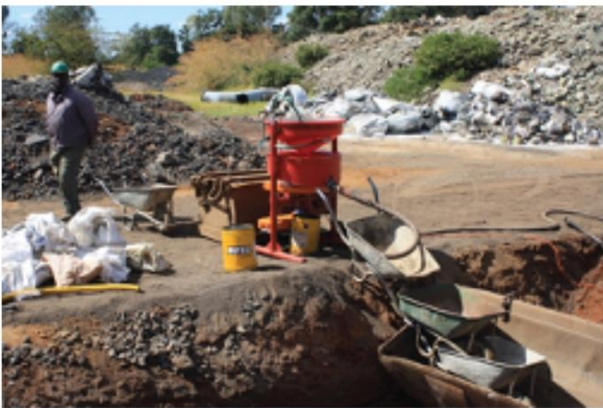
Feeding the GoldKacha with bagged ore feed
