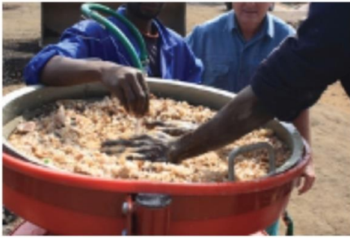
The milled ore being screened and fed into the bowl below by running water
