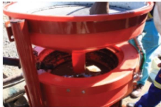
The stationary centrifuge, with concentrate packed in the ribs.
