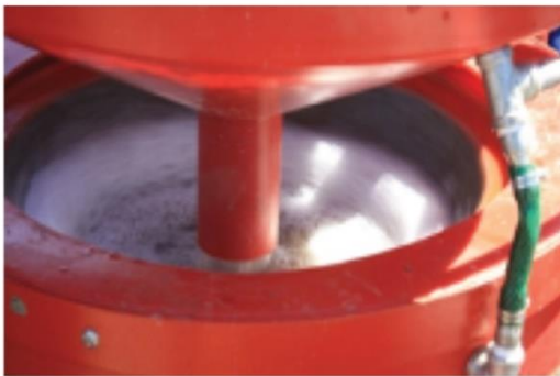
The centrifuge bowl spinning, bubbles from the liquid soap.
