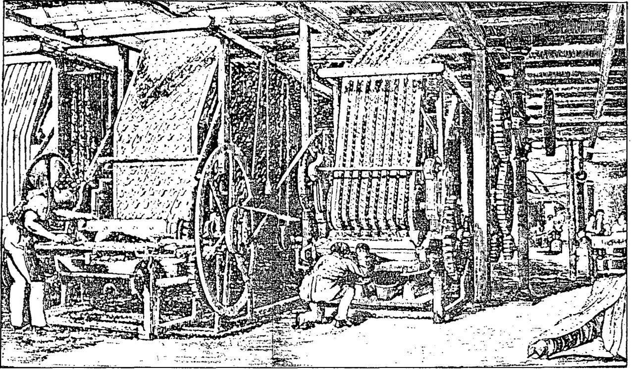
Interior of an early printworks showing wooden-framed machines working in conjunction with blocking tables. This illustration from G S White's Memoirs of Samuel Slater, Philadelphia, 1836 is a woodcut copy of Allom's engraving for E Baine's History of the Cotton Manufacture in Great Britain, 1835. Judging by the clothing of the operatives Allom's illustration could be of about 1820. The later version here has contemporary clothing.
