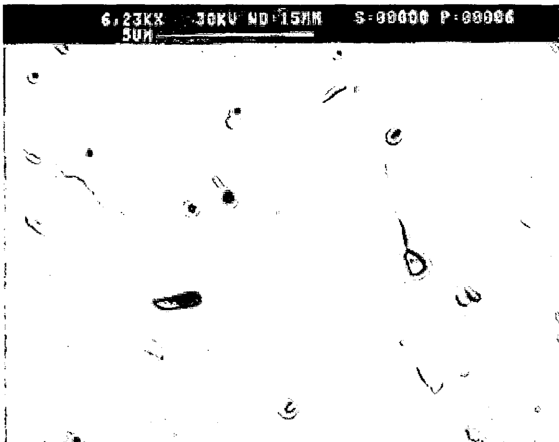
Figure F30 TiO 2 plastic-ceramic fired at 1550°C
