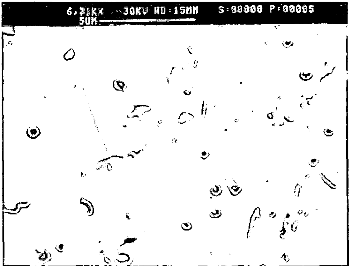
Figure F29 TiO 2 plastic-ceramic fired at 1450°C
