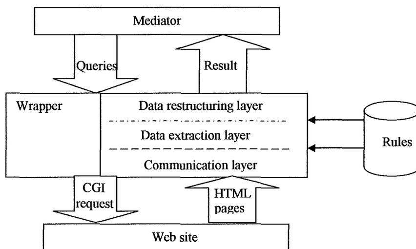
**Figure 6.5. A general architecture of a web wrapper.**
