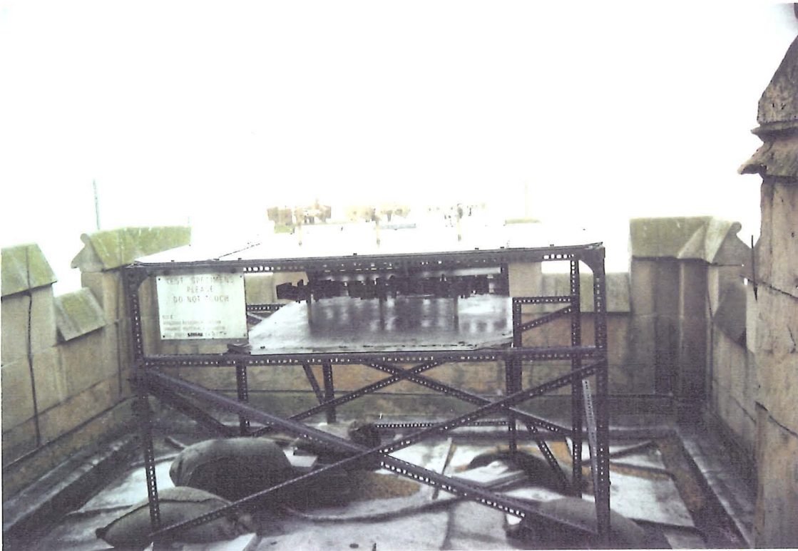
Plate 2.6 Sampling rig used to support stone carousels at Bolsover Castle
