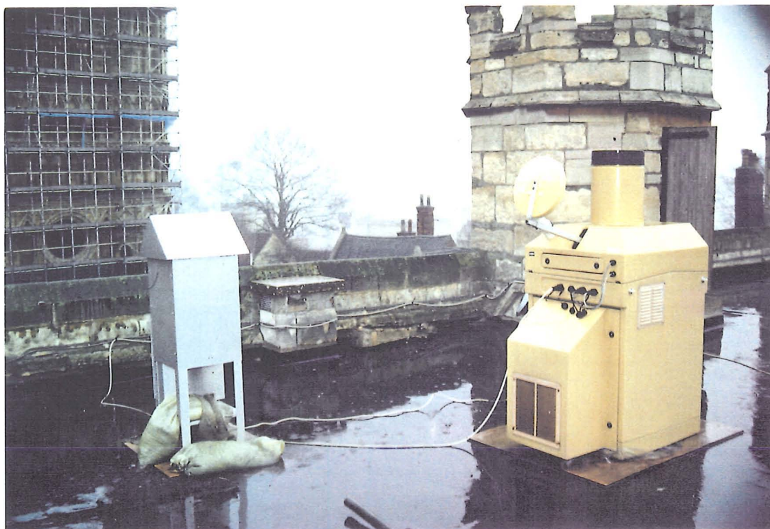
Plate 4.2 (a) Positioning of the high volume sampler on the roof of the Exchequer Gate, Lincoln.
