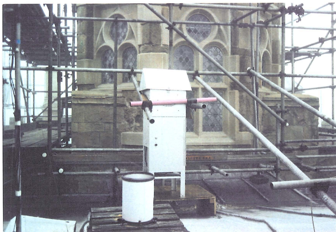
Plate 4.2 (b) Positioning of the high volume sampler on the roof of Bolsover Castle.
