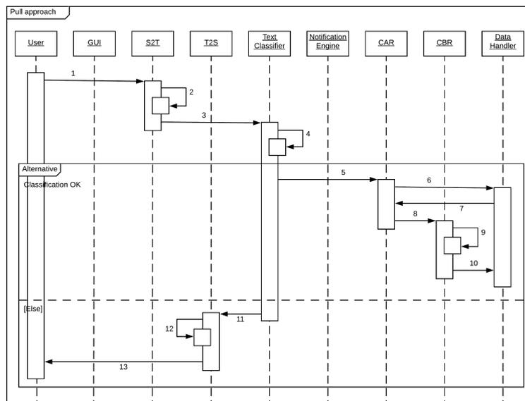
Figure 4.11: Sequence diagram: pull approach
