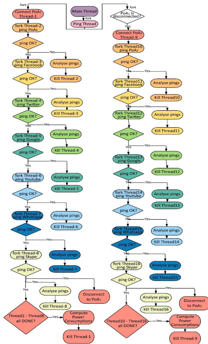
Figure 5. Multi-threaded flowchart of the proposed ping transmissions when there are two available APs.
