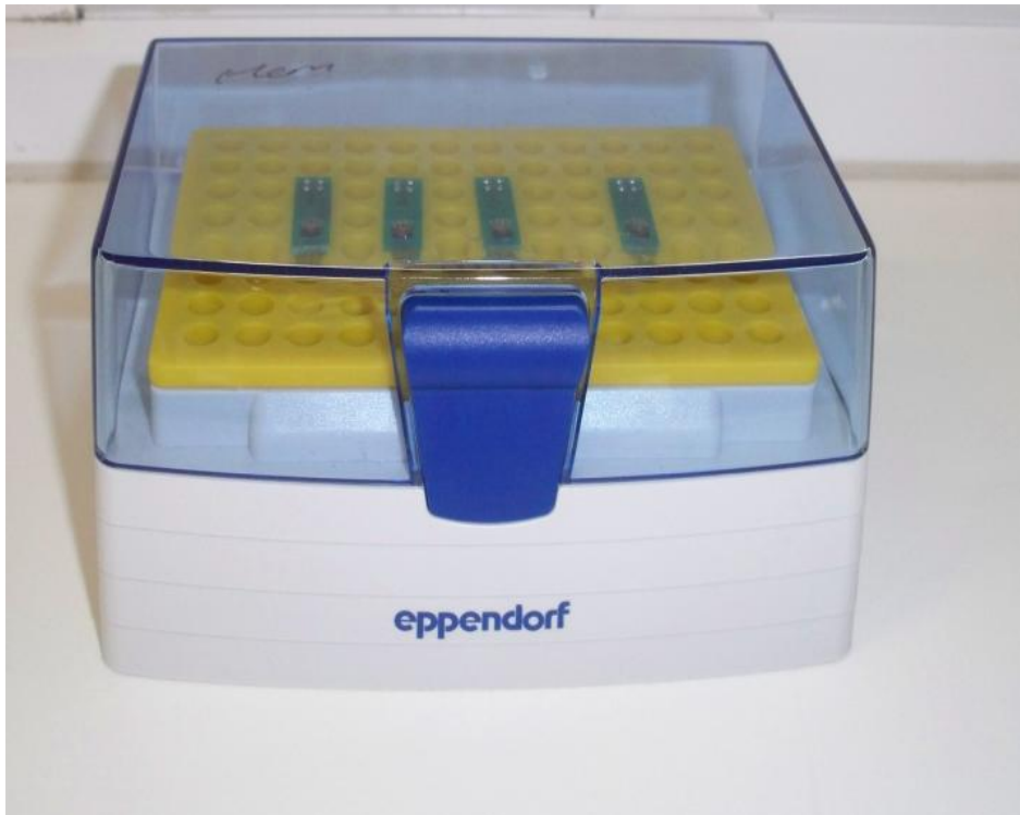
Figure 3.2: Humidified chamber into which biosensors were incubated at every stage in their construction.
