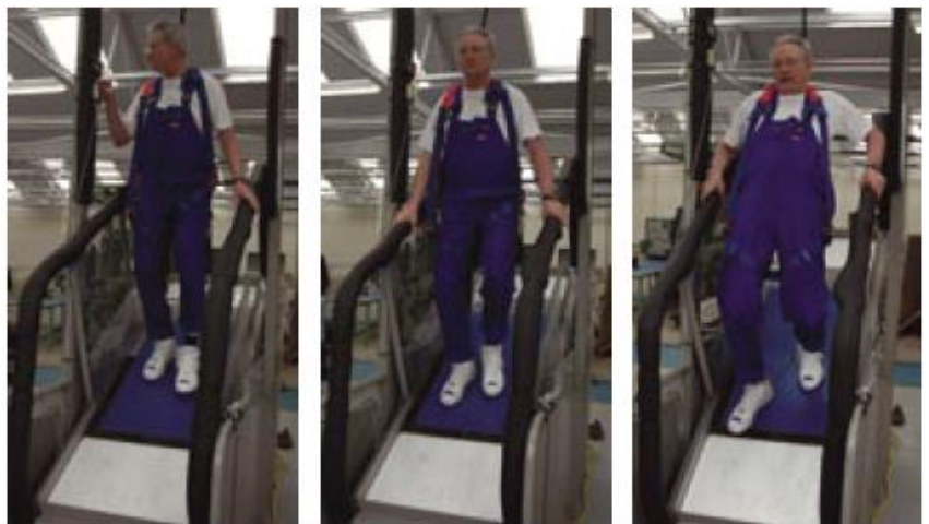
3.7 DIN Ramp test being undertaken at CERAM Research Ltd.
