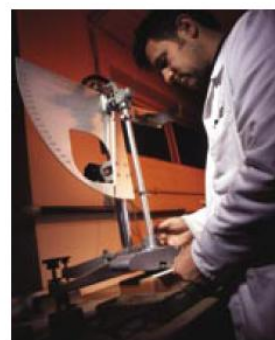
3.6 Pendulum test being undertaken at CERAM Research Ltd.
