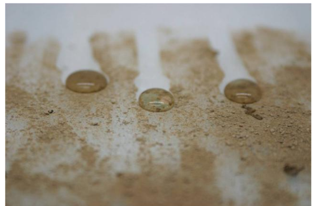
8.3 Detail of self-cleaning glass
