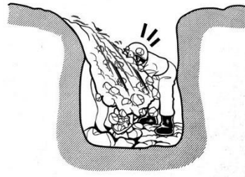
d) Hazard 4 (H4): Collapse of foundation pits
