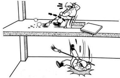
b) Hazard 2 (H2): Fall from uncovered holes
