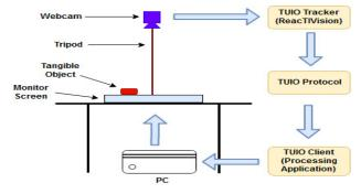
Fig. 4. Hardware setup and software architecture used for TangiNet
