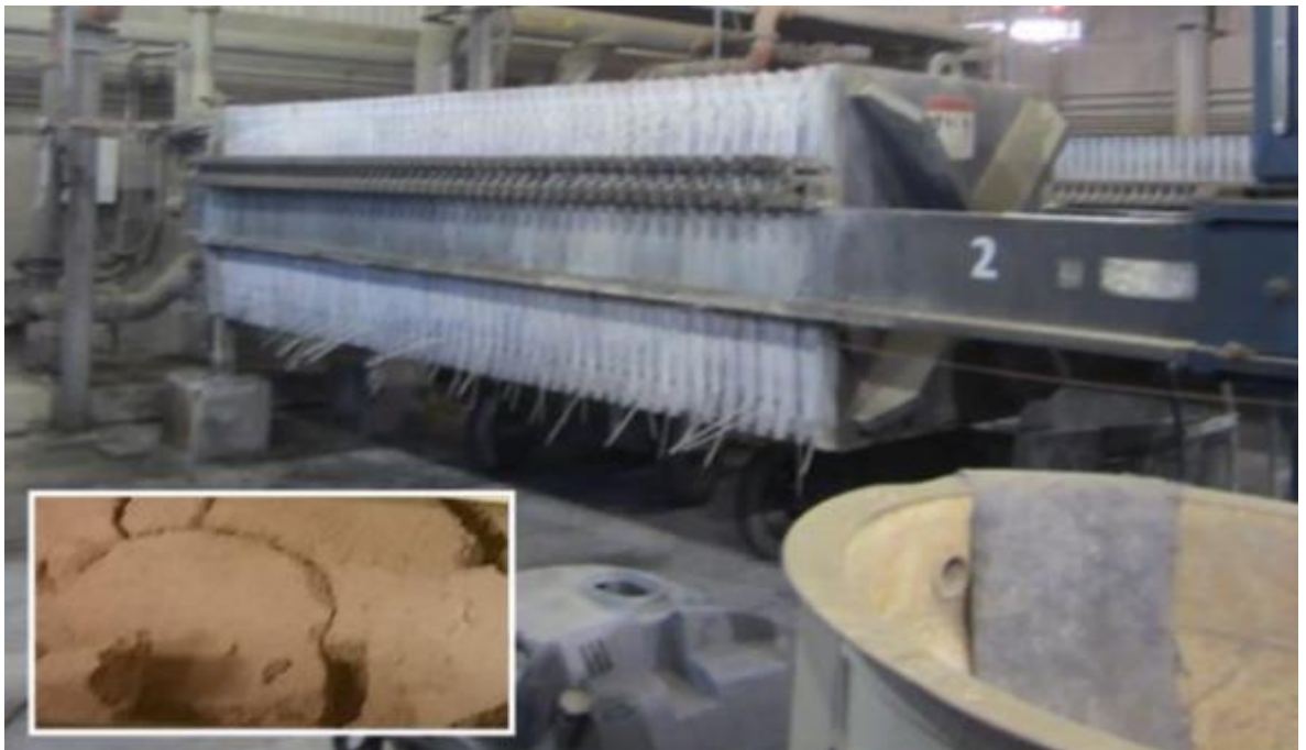
Figure 24: Filtration & Precipitate Production
