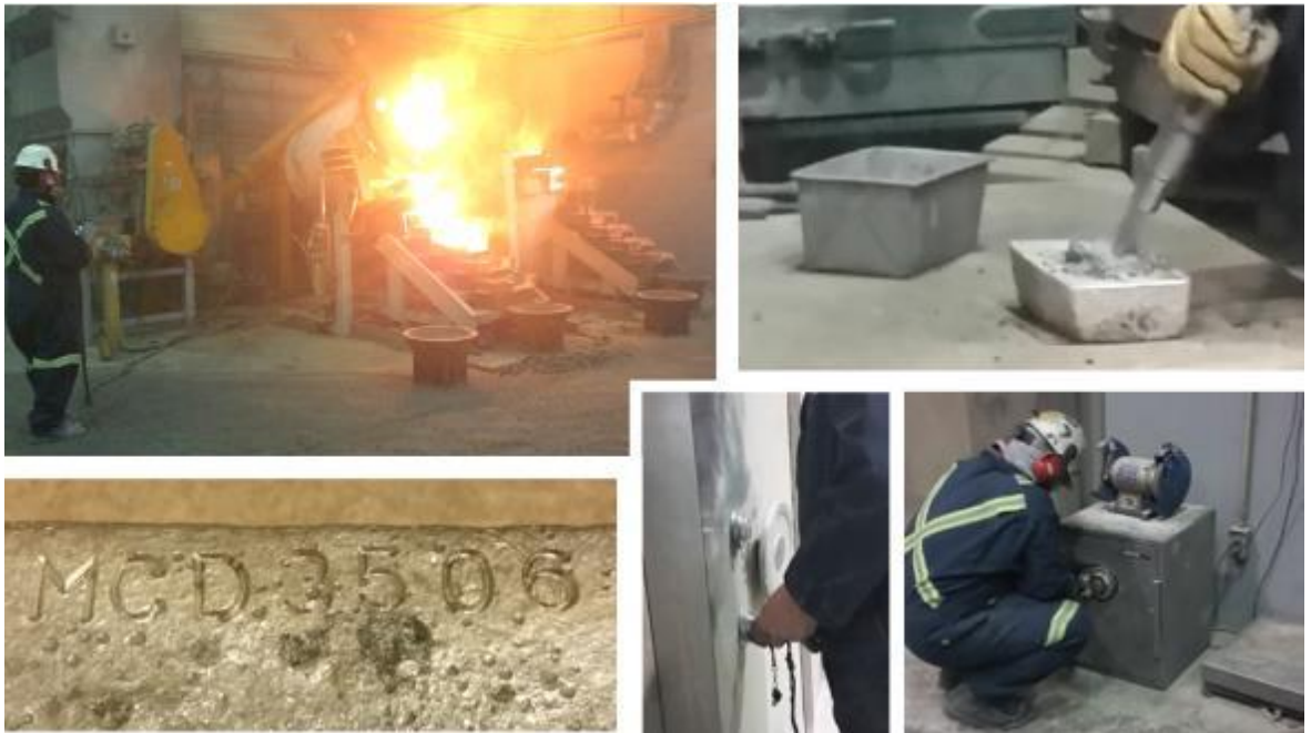
Figure 15: Production & storage of Doré bars
