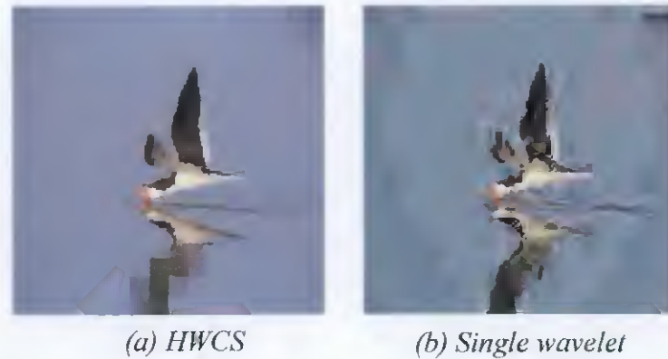
Figure 7.26 Comparison of encoder output for fixed PSNR value
