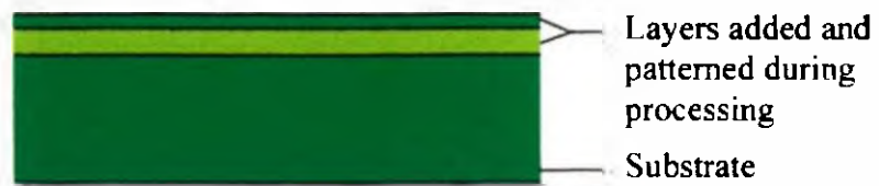
Figure 2.2 Diaphragm Formed by Surface Micromachining
