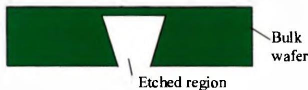
Figure 2.1 Diaphragm Formed by Bulk Micromachining
