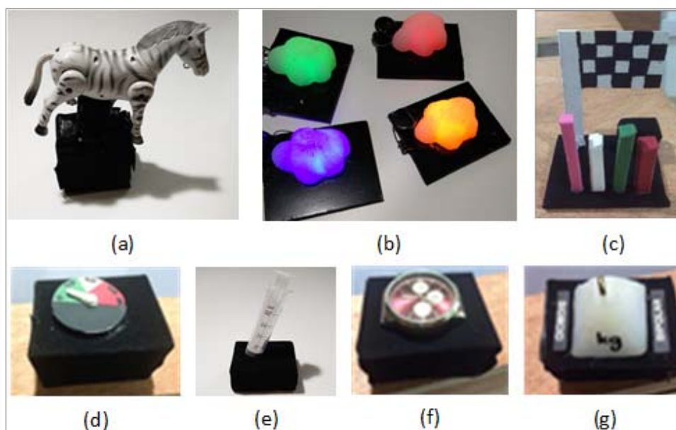
Figure 5.54 Active tangible objects contextualized for ANN operations including; a) Horse - Context Simulator Controller, b) Clouds – Hidden Layer nodes, c) Finish Podium – Output Visualisation, d) Speedometer – Input Speed Value, e) Syringe – Input Health Value, f) Chronograph – Output Time Value, g) Weight – Synapse Weight Adjustment
