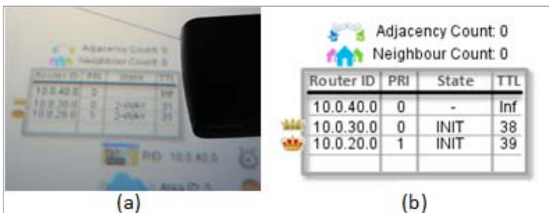
Figure 5.5: Topological tables virtually embodied with physical router illustrate internal data held by the device for OSPF execution.
