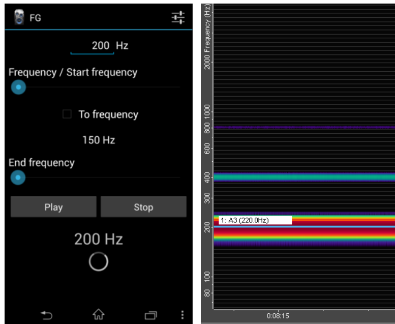
Figure 18: On the left - screen shot of a mobile application that plays a 200Hz tune. On the right - screen shot of the Overtone Analyser accepted result
