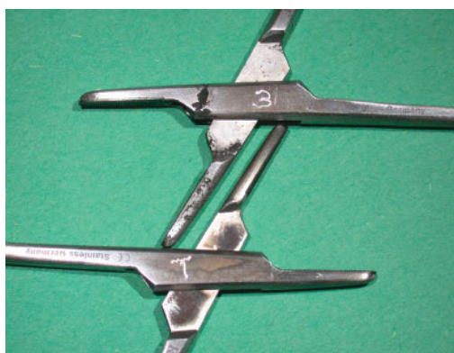
Fig. 1.7: Mayo–Hager carbide-faced needle holders showing severe corrosion and blackening after immersion in bleach for 1 h (The instrument on the top, labeled 3), and autoclaving five times in 1N NaOH (The instrument below, labeled T) respectively (Brown et al , 2005).
