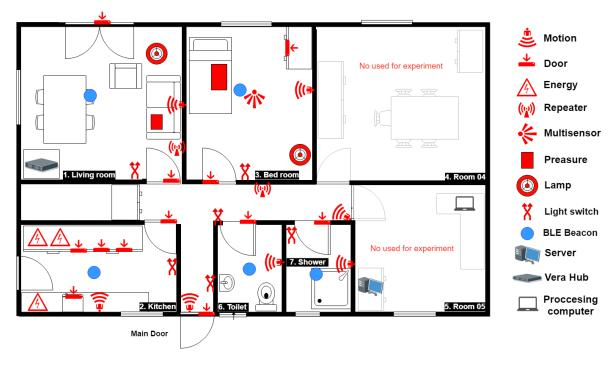
Figure 2. Smart Spaces Lab Layout
