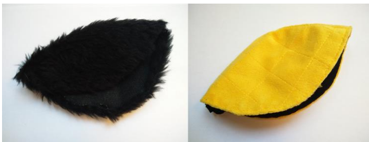
Figure 4.4: The two different covers. Left – synthetic fur. Right – Polyester Fleece
