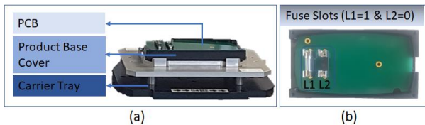
Figure 5. Product Base Carrier Tray (a) Product state after station 2 (b) Top view of PCB with fuse slots
