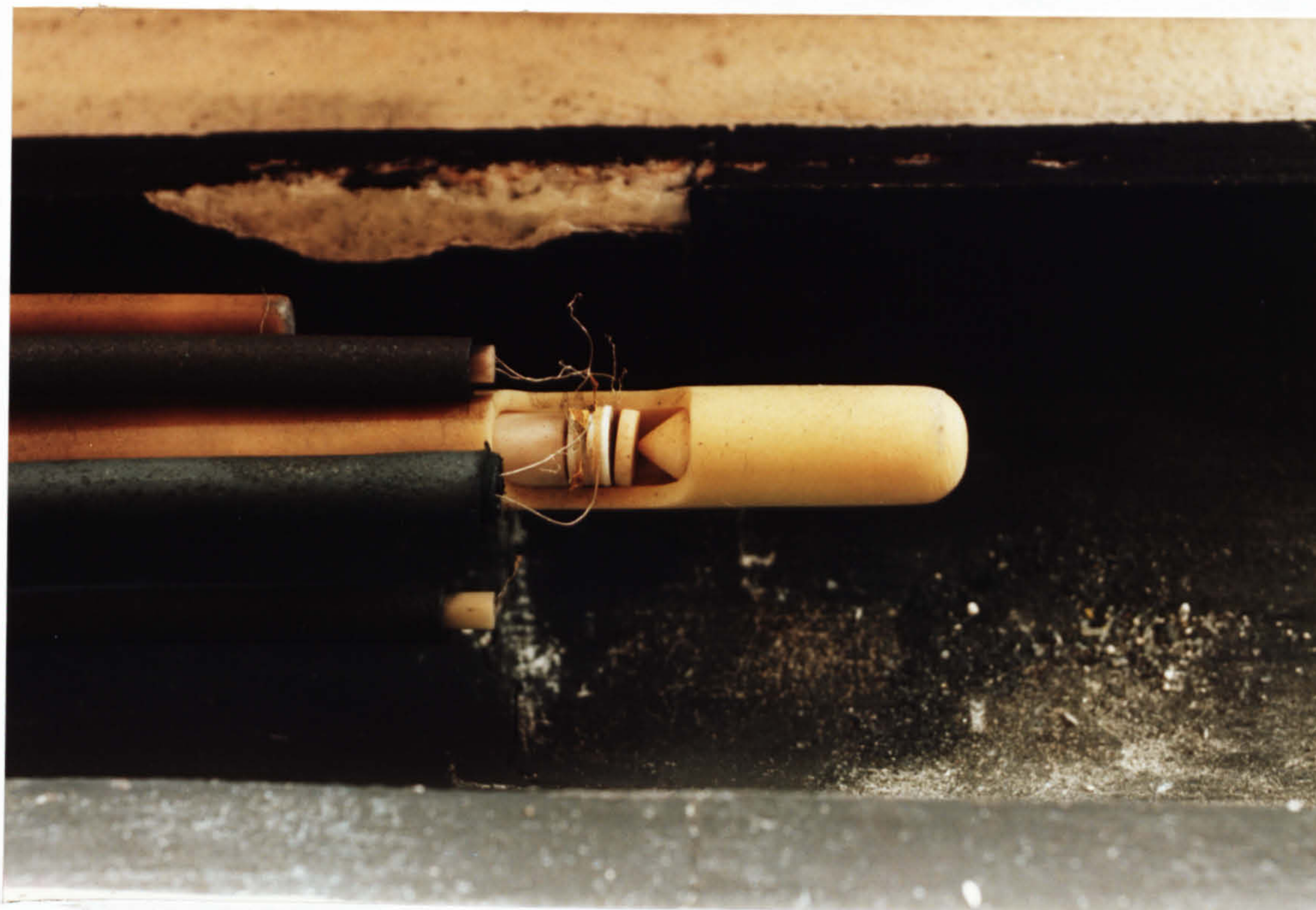
Fig. 2.4: Photograph of a sensor in position for mounting in the rig and connecting with the platinum wires emerging from the shielded tubes. The lower tube is the thermocouple and top tube is a sealed zirconia tube used as a potentiometric sensor.
