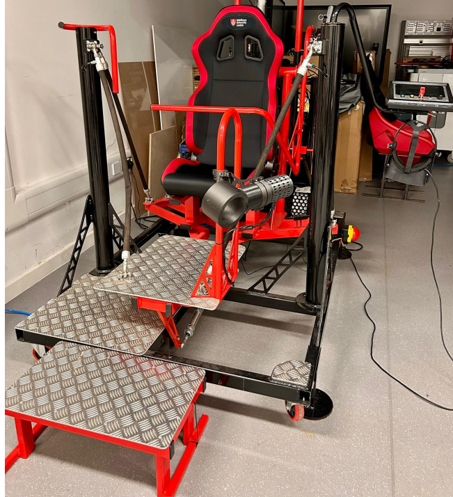
Fig. 1. The VR rollercoaster is powered by a compressor-driven system linked to a Meta Quest visor, which is able to simulate the sound and provide the roller coaster video experience. There is also a fan to simulate the air of the roller coaster.
