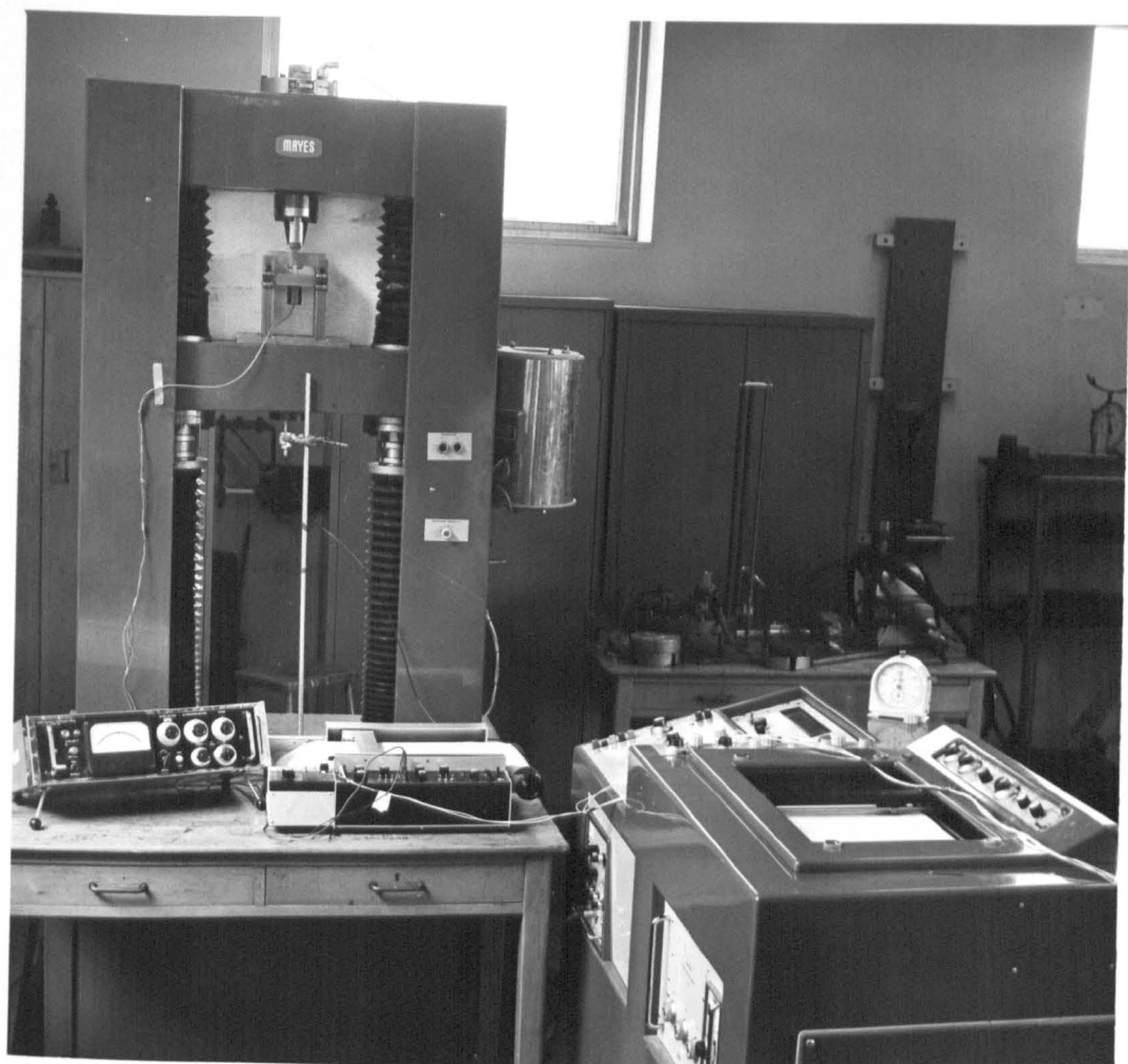
Plate 11.3. Photograph gives the general arrangement and the equipment used for the three-point bend test with COD measurement.
