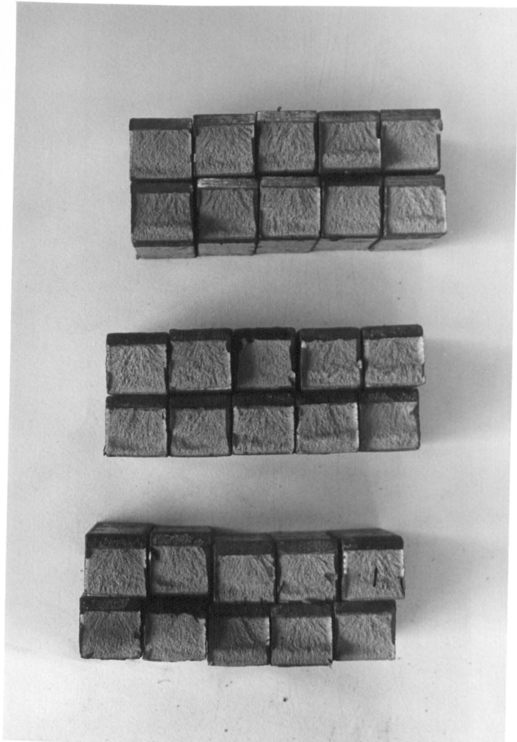
Plate 11.9. Light fractograph of the EN 8 steel Charpy impact test specimens, placed in a corrosive environment, NACE solution with H 2 S (1 atm.) at 60° C, for 750 hours and tested in air at room-25 ± 2° C. It shows much coarser fracture surface and very little deformation in all the specimens.
