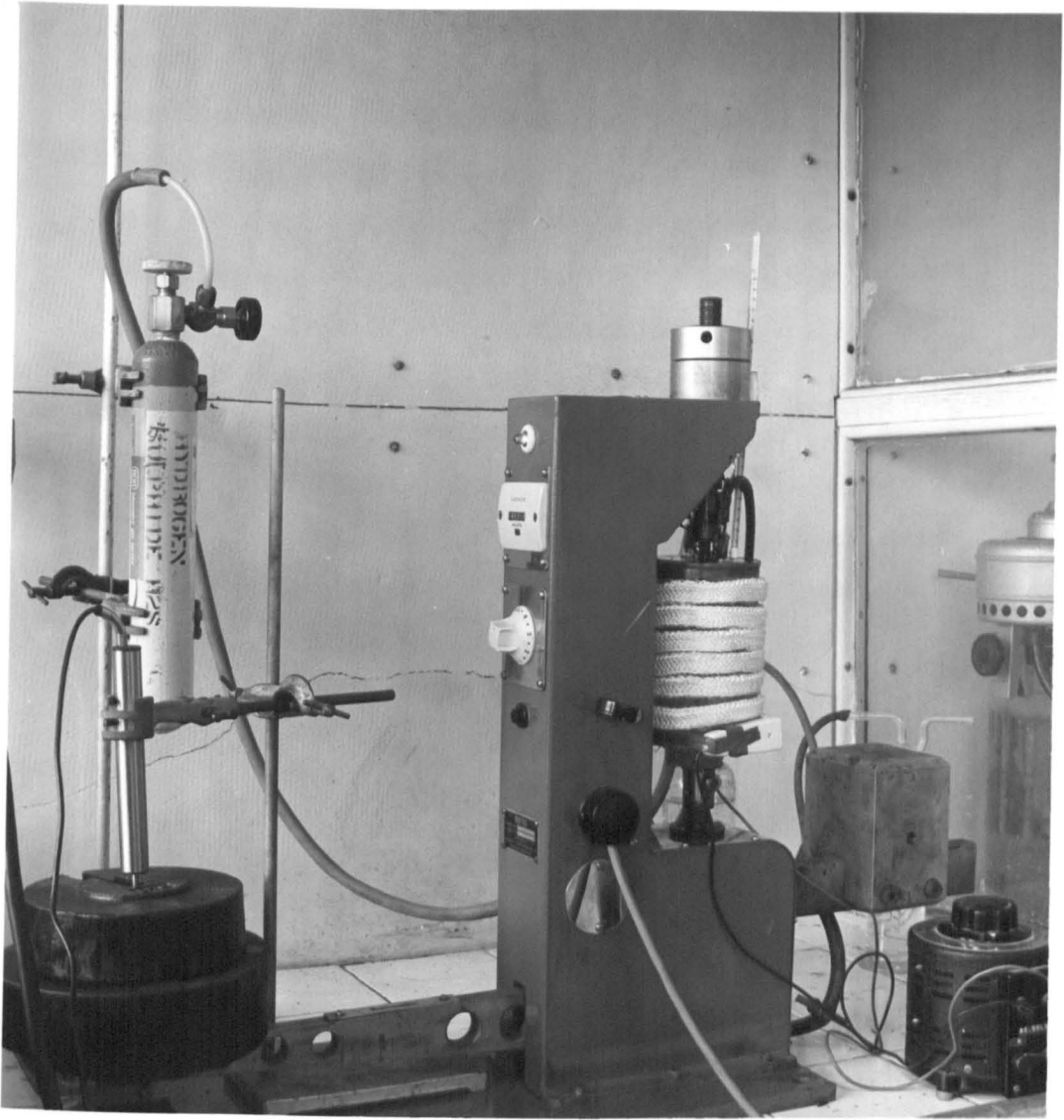
Plate 10.1. Photograph of a sustained load test set-up.
