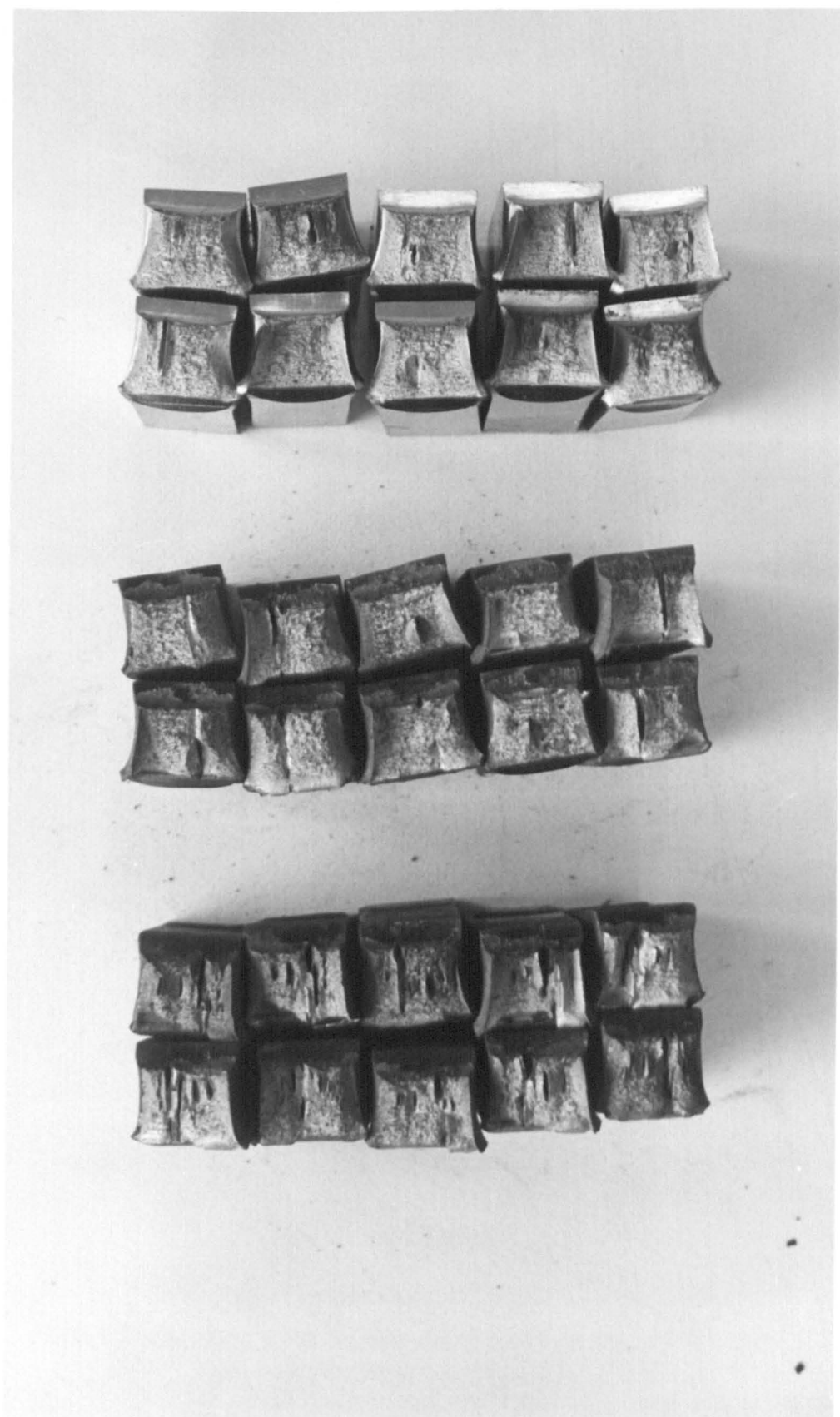
Plate 11.14. Light fractograph of the API 5LX 65 pipe-steel Charpy impact test specimens, placed in a corrosive environment, NACE solution with \text{H}_2\text{S} (1 atm.) at 60^\circ\text{C} for 850 hours and tested in air at 20 \pm 2^\circ\text{C} . It shows some blister type attack on unprotected specimens and a comparison of specimens' deformation among the three types.
