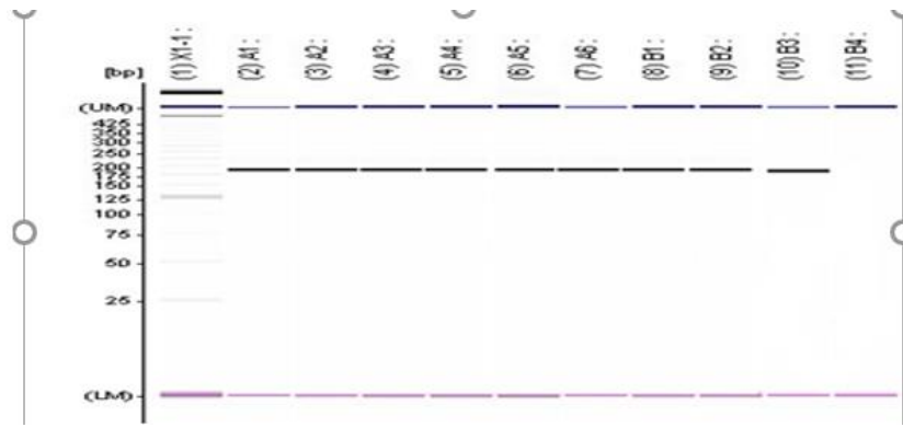
Figure 32: Results of malaria parasite analysis by MultiNA. PCR products are represented in lanes (A1-B2) are 205bp in size. B3 and B4 refer to positive and negative PCR controls; respectively. X1-1 represents 25 bp markers used.
