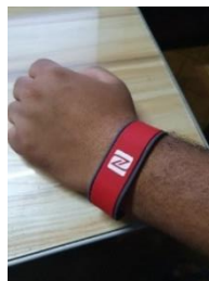
Fig. 2. NFC Chip embedded in Silicone Bracelet
