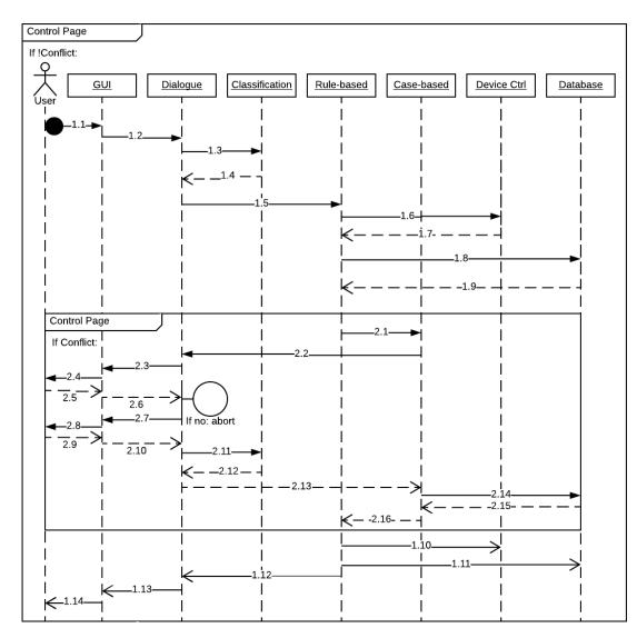
Fig. 5. UML Sequence diagram of the system
