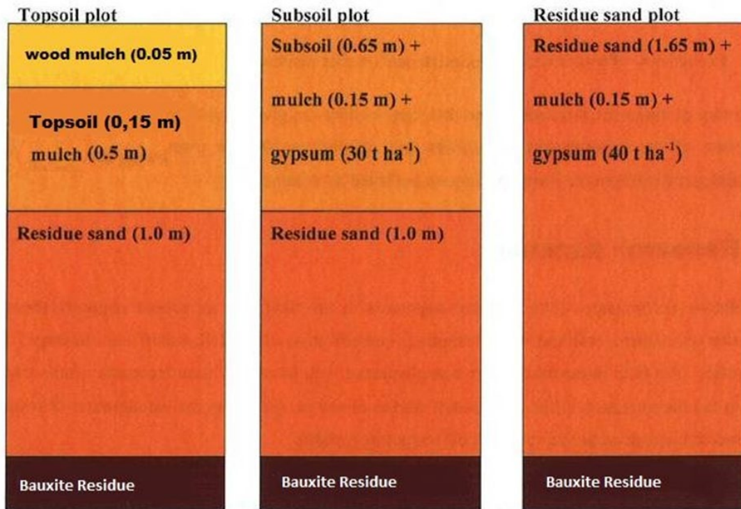
Figure 24 Schematic presentation of the three capping sequences evaluated at the B.R.D.A. in Alcan Gove, Australia
