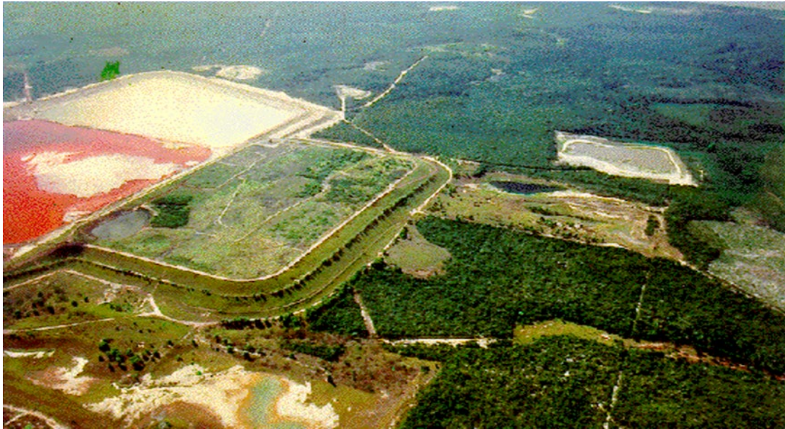
Figure 14 Alumar residue disposal area #1 surface in September 1998. Note that area is almost blended with surrounding vegetation.
